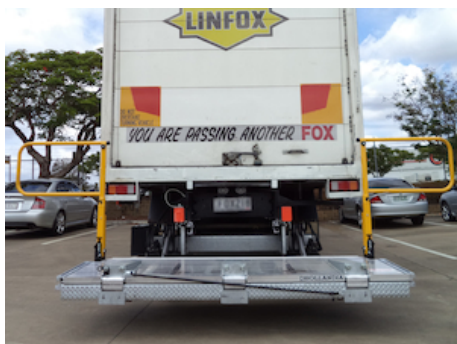
OAP204.LR - 2 safety rails with rotating foot
