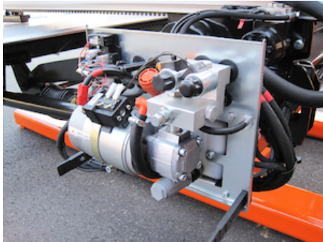
Pump unit 12V or 24V DC, accessible on 5 sides for easy maintenance
