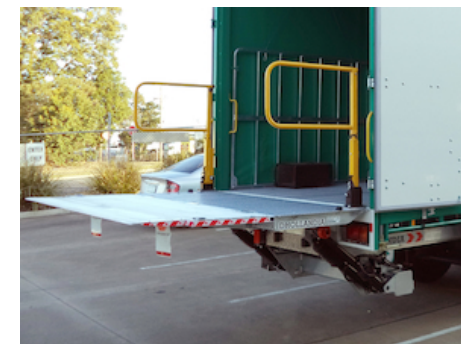
OAP203.LR - 2 hinged safety rails on foldable platform
