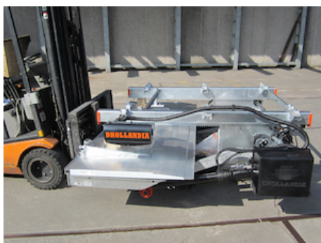
OAM100 - Premounting of slider lift
