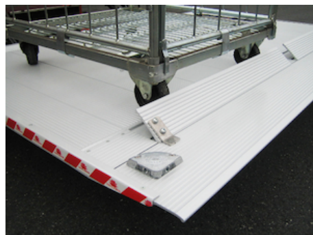
OAP100.M - Manual rollstops in platform point
